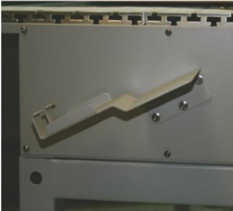
Step 3 - Mount Pendant Holder and re-install nuts
