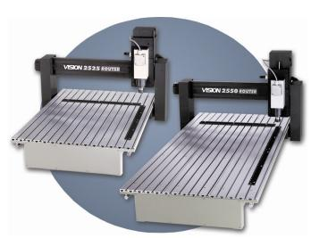
25" x 50" work areas. These larger table sizes allow users to cut out sheets of acrylic, particle board, aluminum, plastics, and other materials in sizes up to 2' x 4'. These machines also include an automatic surface-setting block and offer 7" of clearance with a higher gantry. Customers may add Vision's new DACS (Digitally Aligned Cutting System) camera, an alignment tool which provides perfect print-to-cut registration for their routers and engravers.
