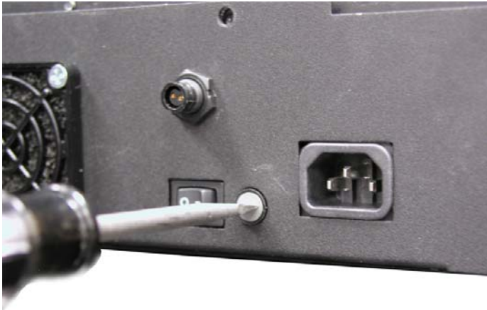
(Figure 5.15) External Fuse removal
