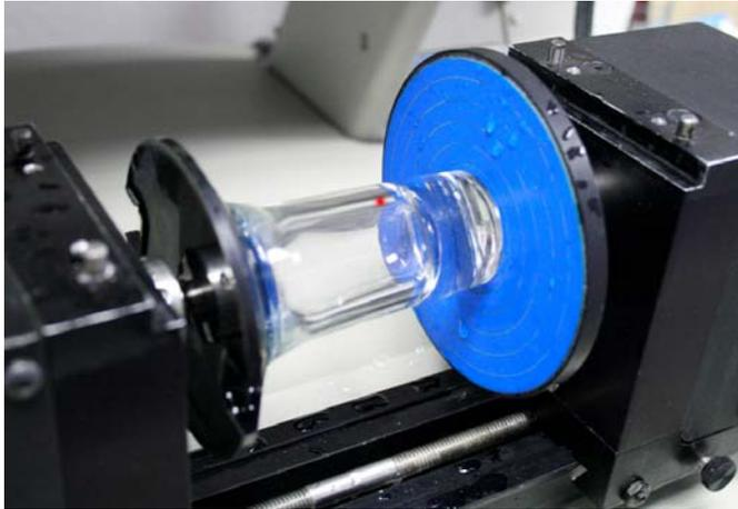
**Step 4/Photo 5:** We then sent the job to the engraver. To keep the image clear and concise, we used an XY feed rate of .4 inches per second, a Z feed rate of .6 inches per second, and a spindle speed of 12,000 RPM. Also, we used the MaxPro's recirculating water system to keep the area we engraved wet. This increases the quality of glass engraving and prolongs the tool life of the rotating diamond. Once finished, we cleaned the debris and water off of the glass material using a paper towel.
