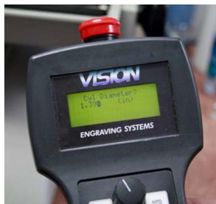
**Step 3/Photo 4:** We then set the engraving area using our "Measure" feature in the Vision Pro 8 software. This allowed us to set home over the center of the area to be engraved.
